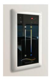
Deblick fixtures are equiped with DALI dim driver and Dynamic Lighting Control. Daylight sensors, attendance sensors, and time sensors are integrated to deliver an optimal lighting rythm. The programmed rhythm can of course be interrupted and resumed at the push of a button.
